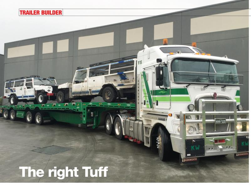
THERE'S NO SUCH THING AS FAVOURITISM AT HOGAN'S HEAVY HAULAGE. TO PUT IT SIMPLY, HAVING THE RIGHT VEHICLE FOR A SPECIFIC TASK WILL ALWAYS BE THE COMPANY'S TOP PRIORITY, WHICH IS WHY IT HAS SELECTED TUFF TRAILERS' QUAD-AXLE TILT 'N' SLIDE DECK WIDENER.
