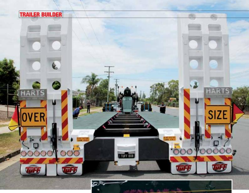
has a central catwalk designed for low height user access, as now often requested in the mining industry. Equally important for safe on-site operation is the patented 'Ezy Lift' tyre carrier at the front. Now capable of carrying up to 12 tyres, it will waive the need to climb the gooseneck and reduce the associated OH&S risk. In addition, all tie downs and load restraints are RUD-certified.
