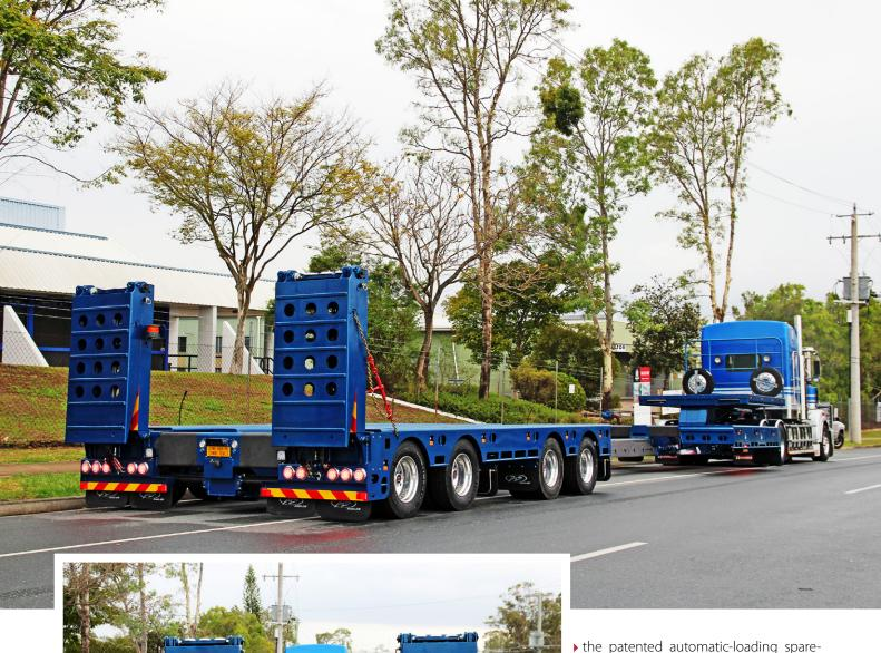
the patented automatic-loading sparetyre carrier, for example, that can be stacked alongside the gooseneck, so the operator does not have to climb up or roll heavy wheels around – a significant saver on the H&S front.
